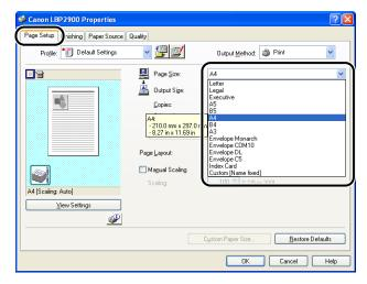
3 Set the [Output Size] setting to the size of the paper loaded in the printer as needed.
